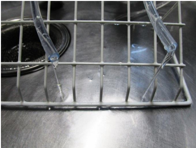
Fig. 3: Adjustment to 20 mL per minute for both circuits (Slight amount of water water leakage)
